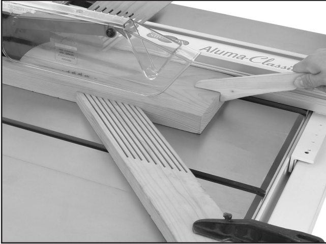
Figure 43. Typical ripping operation.
